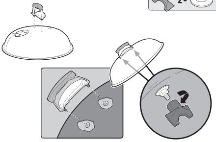
Tighten hardware until it is secure.
