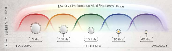
\* 20 kHz and 40 kHz not available as single operating frequencies in EQUINOX 600. Multi-IQ frequency range shown applies to both EQUINOX 600 and 800. This diagram is representative only. Actual sensitivity levels will depend upon target types and sizes, ground conditions and detector settings.
