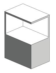
In the case of balconies, at least 20% of the total of the side, back and front wall areas shall be and remain open and unrestricted.
