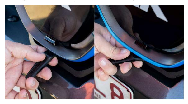
Attaching the accent ring is just as easy, however you'll first want to make sure the ring is in the right orientation. On the back of the accent ring is a T-shaped tab. Position the T-shaped tab at the bottom of the ring, and align it with the slot on the bottom of the light housing. Push the rest of the ring onto the light from bottom to top to attach the ring.
