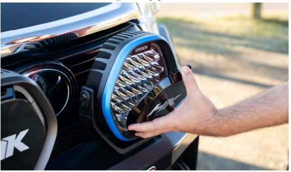
To attach the cover, align the tabs on the bottom of the cover with the corresponding slots at the bottom of the light. Push the top of the cover into the light until you hear a click. This is the top tabs snapping into place.
