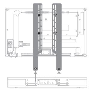
Use screws to fix the soundbar bracket behind the TV, then use 2 pcs M4\*10 screws to fix the soundbar
