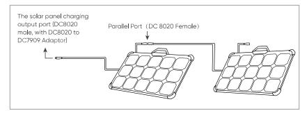
Tip: Users can enter the number of solar panels in their own combination according to the number of solar panels they purchased. Currently, the product supports charging with 1, 2, 3, 4, 6, 8, and 12 80W solar panels in combination.
