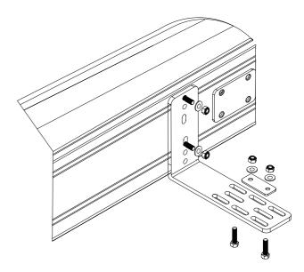
You must ensure the bracket you use is supported by either the roof rack or other form of support.
