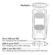
A USB charger is required to charge the powerbank. This can be a wall charger, a car USB charger or any USB powered port.
