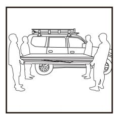
With no less than four people, lift the rooftop tent onto the roof platform. Make sure the main door is facing backwards from the vehicle before attempting the lift. Centre the tent ensuring the weight is distributed evenly. Ensure the rear of the tent is flush with the vehicle so the ladder can be fitted.
