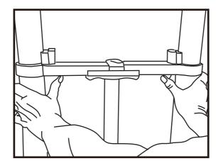
3. To close the ladder, grasp with both hands and press the left and right switches on the lowest cross piece. Slowly collapse the ladder in the opposite sequence to opening it.
