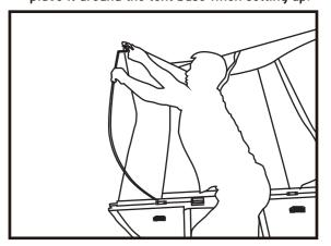
3. Set up the awning with two spring poles. Insert the straight end to the bracket on the base and the other end to the hook on the awning.
