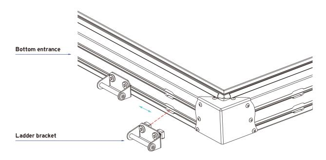
Slide the two ladder brackets into the slot on the base. Secure the screws with the Allen key provided.
