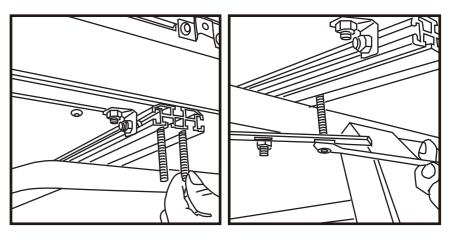
Secure each of the four corners with the brackets and screws provided. Each mounting point requires two 55mm M8 screws that slide into the slots on the mounting bar. Tighten the Nyloc with washer using the spanner provided.
