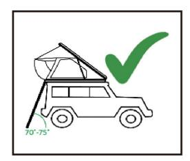
Adjust the length of the ladder to make sure the angle is approximately 75 degrees between the ladder and the ground.
