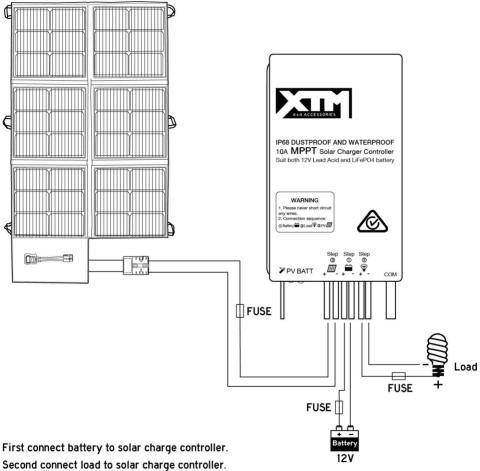
Finally connect solar blanket to solar charge controller.
