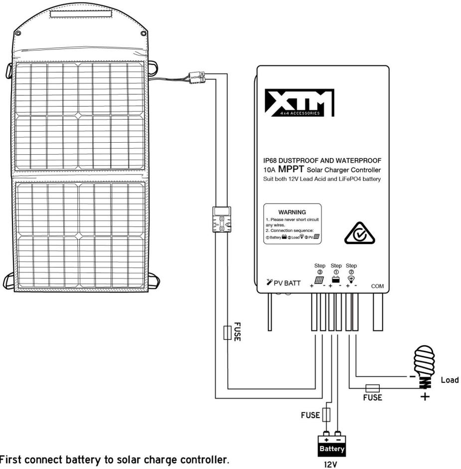
First connect battery to solar charge controller.
