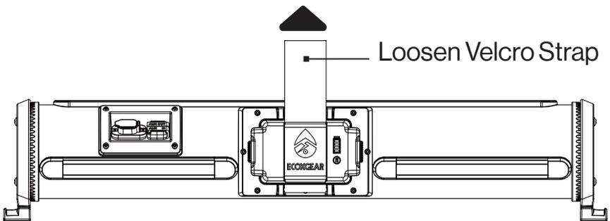
2. Loosen the velcro strap that is fastened over the Battery Pack.
