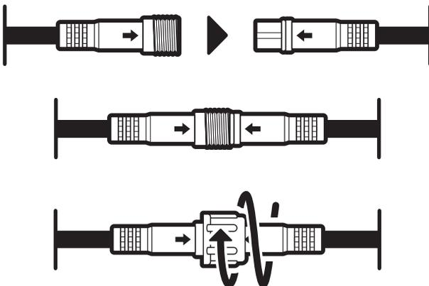
3. Connect the 3-pin female connector on the Deutsch LED Cable to the 3-pin male connector on an LEDCast-enabled product. Align the arrow on both connectors, push in and screw the nut cap on the female connector.
