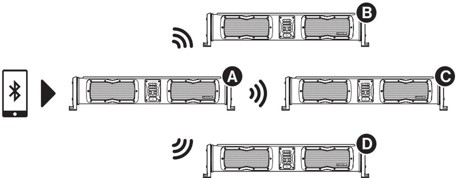
1. Turn on the additional EcoCast-enabled speakers (**Speaker C** and **Speaker D**) and press the Audio Mode Button to cycle through to and initiate EcoCast Receiving Mode. The Mode LED Status Indicator will flash Green, and the speaker will announce, "EcoCast receiving."
