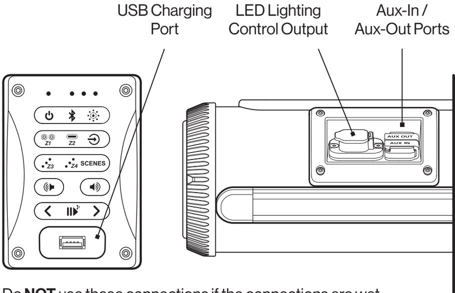
Do **NOT** use these connections if the connections are wet.
