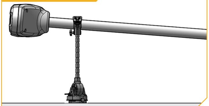
holes, and install screws. It may be necessary to shim or modify the deck or gunwale under the mounting location to create a flat area for the base to be mounted.
