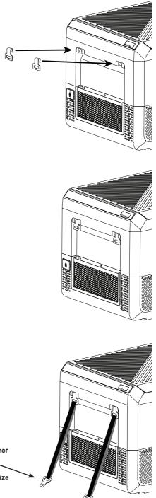
Tie-down straps and lower anchor points/fridge slide need to be sourced separately and sized appropriately from the fridge size
