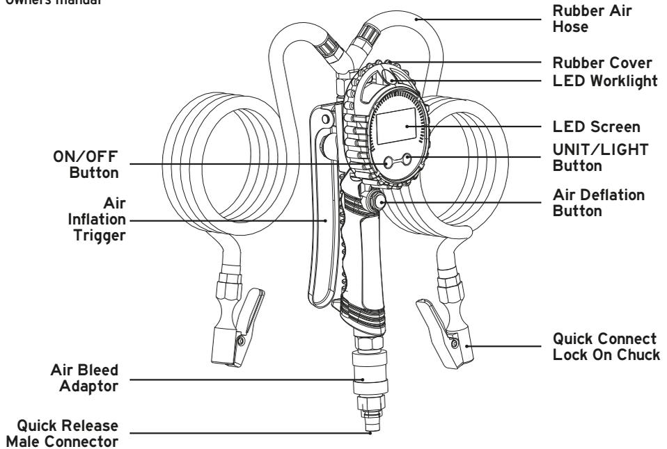
**Air Bleed Adaptor: Push UP to release air from air compressor
