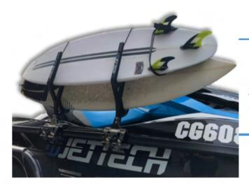
For a 6ft Surfboard space the racks approximately 60-80cm apart from each other sitting in the middle of the ski. The rack posts are shaped and profiled for surfboards to slot in with the top - waxed sides facing each other and fins at opposite ends. We suggest always putting the larger board in the bottom slot.
