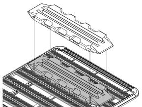
6 Lock the track in place by rotating all 4 knobs clockwise until it is tightened. Confirm by giving the tracks a small shake and make adjustments if required.
