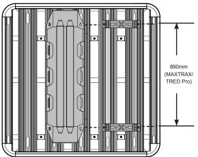
Note: For sideways mount, adjustments to the three slotted tray mounting holes may be needed to achieve the required mounting distance.
