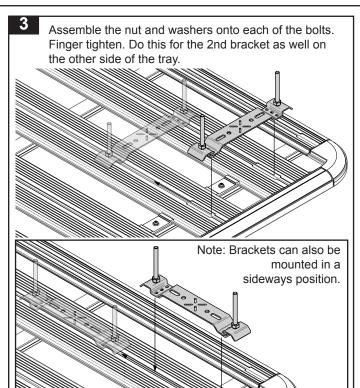
Adjust so the brackets are in the correct mounting distance apart to suit the recovery track by placing the track on the side as a guide. A MAXTRAX and TRED Pro would require a distance of 890mm apart as shown below.
