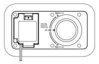
3. Turn the control dial counter-clockwise to the "Off' position upon reaching desired firmness. Make sure the switch aligns with the "Off' arrow. Airbed is now ready for use.
