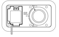
2. Turn the control dial clockwise to the "Inflate" position to inflate the air bed.
