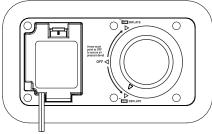
1. Turn the control dial counter-clockwise to the deflate position for complete deflation.
