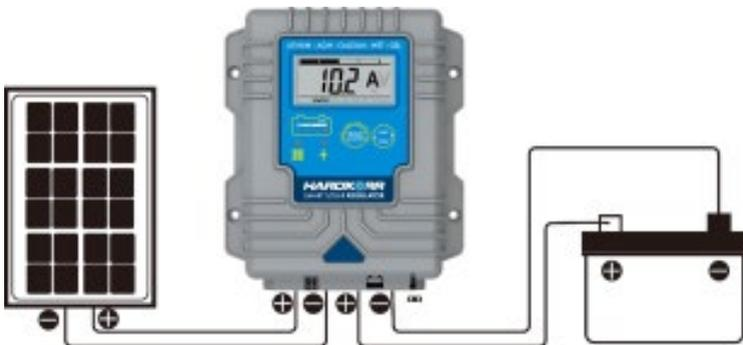
Please check your battery manufacturer’s specifications to select correct battery type. The unit has charge programs for six different battery types: Lithium Iron Phosphate (LiFePO4), Lithium Titanate Oxide (Li4Ti5O12), Gel, AGM, Wet and Calcium.
