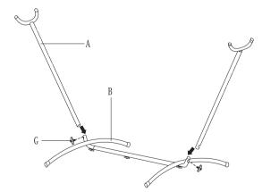
Install the perpendicular struts (A) on the foundation struts (B), align the individual parts of the frame so that overlap the attachment bolt holes (G) and tighten the joint sufficiently. Repeat the same procedure on the other end, see the figure above. Align the parts so the holes line up. Insert the bolts, nuts and washers.
