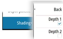
In the following example water depth from 5 meters to 10 meters will be shaded yellow in the chart when Depth 1 is the selected shading in the menu.
