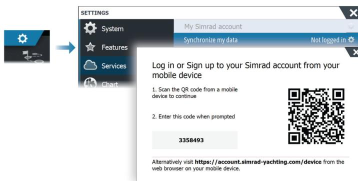
2. Use your mobile device to scan the QR code® which displays on the login page, or open a web browser on your mobile device and manually enter the web address listed on the MFD.
