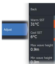
You can define the Sea Surface Temperature (SST) range and wave height color coding. The temperature above warm and below cool values is displayed as progressively darker red and darker blue.
