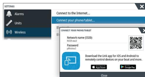
The MFD network name (SSID) will be displayed as an available network in the phone/tablet.
