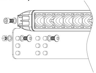
Place the spring washers on the Hexagon socket round head bolts, then insert the bolts through the plate mounting bracket and the back hole on the light bar. Tighten all until the light holds position.
