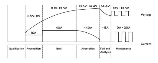
Charging algorithm will change according to battery type.
