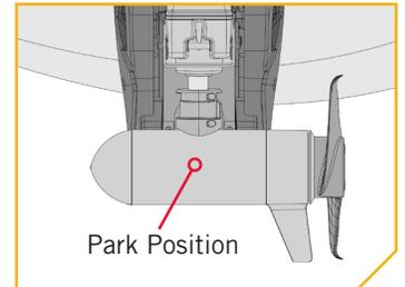
**NOTICE:** If the motor was stowed with the prop pointing up or down, you may need to depress the button on the left front motor ramp to deploy the motor. Release that button when the motor starts to deploy.
