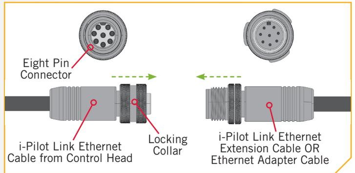
**NOTICE:** The connectors are keyed to prevent reversed installation.
