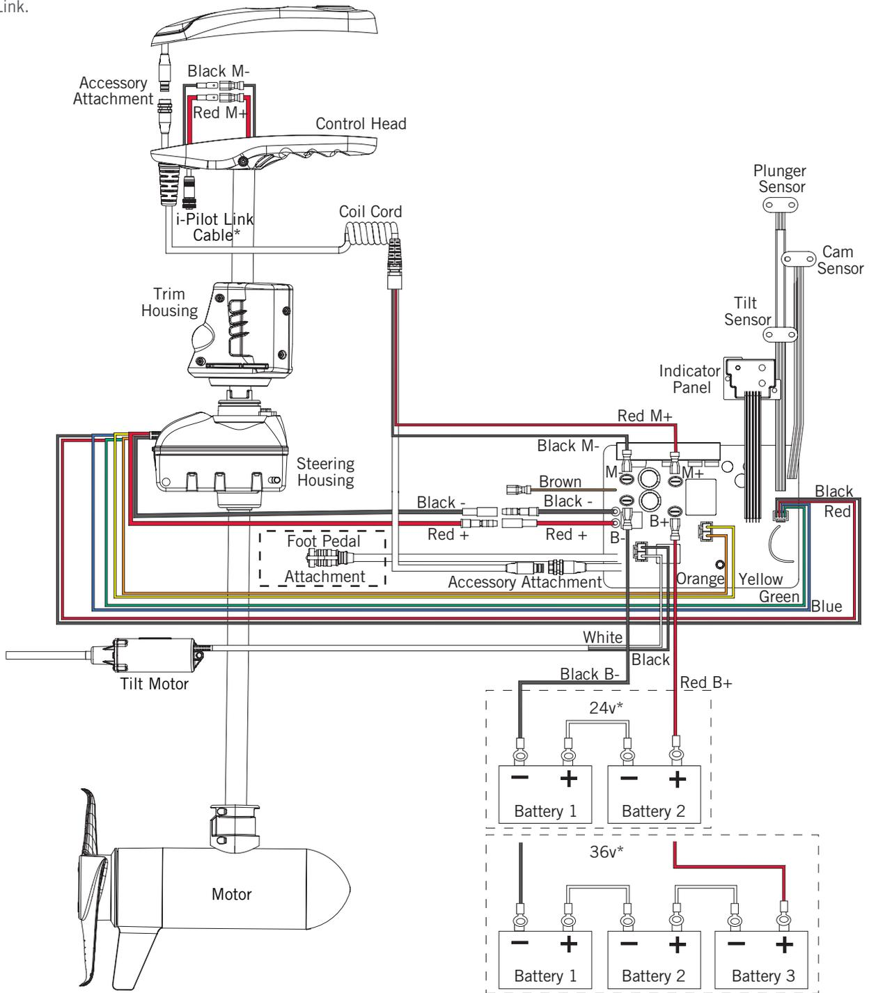
**NOTICE:** This is a multi-voltage diagram. Double-check your motor's voltage for proper connections. Over-Current Protection Devices are not shown in this illustration. \*i-Pilot Link Cable attachment for i-Pilot Link only.
