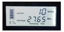
If an AC adaptor is also connected to the input, the screen will display the net amount of watts and the current charging status.
