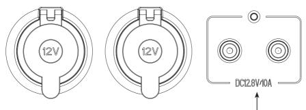
NOTE: There are 2x DC5521 adaptors included to allow use of most LED strip lighting directly  ${\sf J}$  from these DC jack outlets
