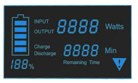
The LCD display will show the total input/output in watts and the remaining time to either charge or discharge. What the LCD screen displays depends on the Input and Output. For example, if two phones are attached, the screen will show the below -
