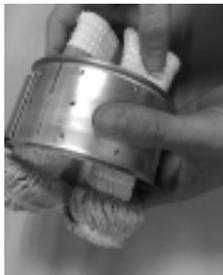
6. Place the wick in the heater and position the control system. The end of the control button must again fit in the slot.
