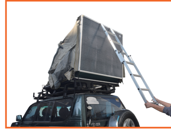
7. Whilst pulling down on the end of the ladder, walk backwards away from the vehicle allowing the tent to unfold.
