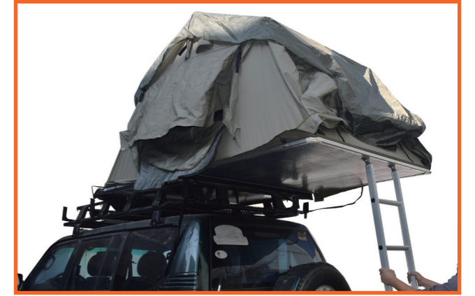
8. When tent is fully unfolded the end of the ladder should touch the ground. NOTE: If your vehicle is too tall to allow the ladder to touch the ground, a ladder extension will be required. See page 12.
