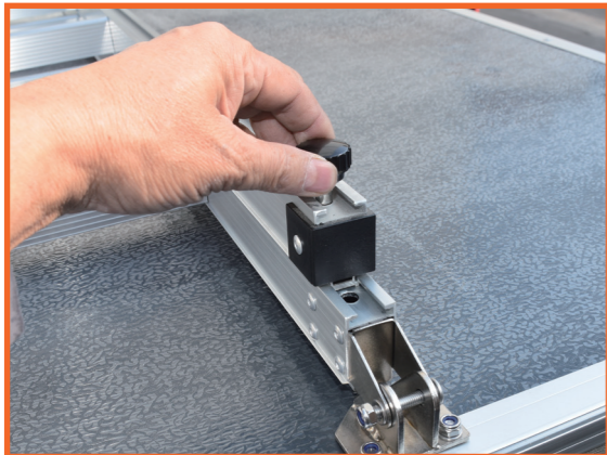
5. The two ladder locking pins require spring pressure to engage them into the locked position. To do this, twist locking pins in an anti-clockwise direction.
