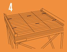
Unfold and place grill grates on top of the rails.
