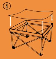
Holding the Fire Mesh with the folded edges facing down, each of the four grommets should be placed over the upright poles of the frame. Take care to not let any one corner drop too far down the uprights.
