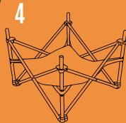
Push down the center of the heat shield and roll the edges to form a bowl shape.
