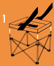
Remove the ashes from your pit. This can be done by either dumping the pit, using a shovel, or by removing the Fire Mesh. To remove the Fire Mesh look for the two bottom Ember Guards from Step 2 of the assembly. Simply place your hands in the middle of each Ember Guard and pull straight up keeping the Ember Guards parallel to the ground. This should remove all four Ember Guards as well as the Fire Mesh as one unit. The Fire Mesh can then be funneled, and the ash dumped out from it
