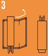
Place the Fire Mesh with the folded side up on the ground. Place the frame and Ember Guard construction on top of the Fire Mesh and roll together tightly. Repeat for Heat Shield if applicable.
