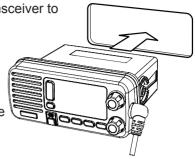
3. Attach the clamps on either side of the transceiver with 2 supplied bolts (5x8 mm). Make sure that the clamps align parallel to the transceiver body.
