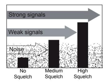
While listening to a channel, adjust the **SQUELCH** knob until the noise is filtered out and you can only hear the transmission. If you switch to a channel with a lot of noise or with a weak transmission, you may need to adjust the squelch level again.
