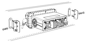
4. Tighten the end bolts on the clamps (rotate clockwise) so that the clamps press firmly against the inside of the instrument control panel.
