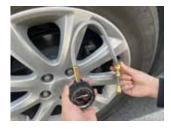
4. Pull back on the slide valve to release air. Push in on the slide valve to stop air, and check the pressure. Note: gauge will not show correct pressure whilst deflating.
