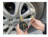
6. Turn the valve stem adaptor anti-clockwise to remove it from the valve stem. Ensure the valve cap is screwed back onto the valve stem.
