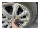
3. Air pressure will push the valve remover out. The gauge will now read the pressure of the tyre.
