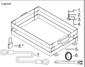
Using item 1,2,3 and 4, install four sets of hardware. Finger tighten.
